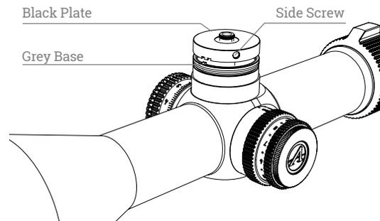
By zeroing the rifle at 100 yards, the shooter can calculate how many clicks of adjustment are needed for different distances or wind conditions. After shooting, the shooter can quickly turn the elevation knob clockwise (down direction) and go back to the zero position once the knob cannot be turned any further. **DO NOT OVERTURN THE ELEVATION KNOB ONCE IT STOPPED.**
