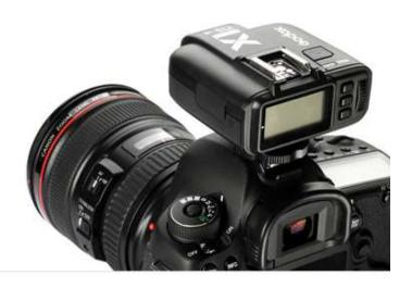
QTII series has built-in Godox 2.4G wireless X system to wireless control multiple Godox flashes (built-in Godox X system) with 16 groups and 32 channels.
