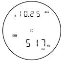
TRIG, a function that is included to support tradesmen and sportsmen alike, displays the true horizontal range and true vertical range, which is based upon trigonometry using angle and line of sight distance. Line of sight distance (LOS) readings will be displayed in the lower portion of the display. The upper display will briefly show the true
