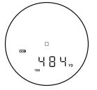
This is the range you will want to use when shooting, rather than the line of sight distance, which may contain gross errors depending upon the shot angle. Readings will be displayed with equivalent horizontal range in the lower portion of the display.
