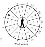
Wind hold values will be displayed in the same output format as elevation; either minute-of-angle (MOA), milliradians (MIL), or inches/cm hold values. TBR/W provides .5 MOA accuracy
