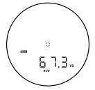
LOS icon will flash indicating the unit has exceeded its maximum BOW range and is displaying line of sight distance only.
